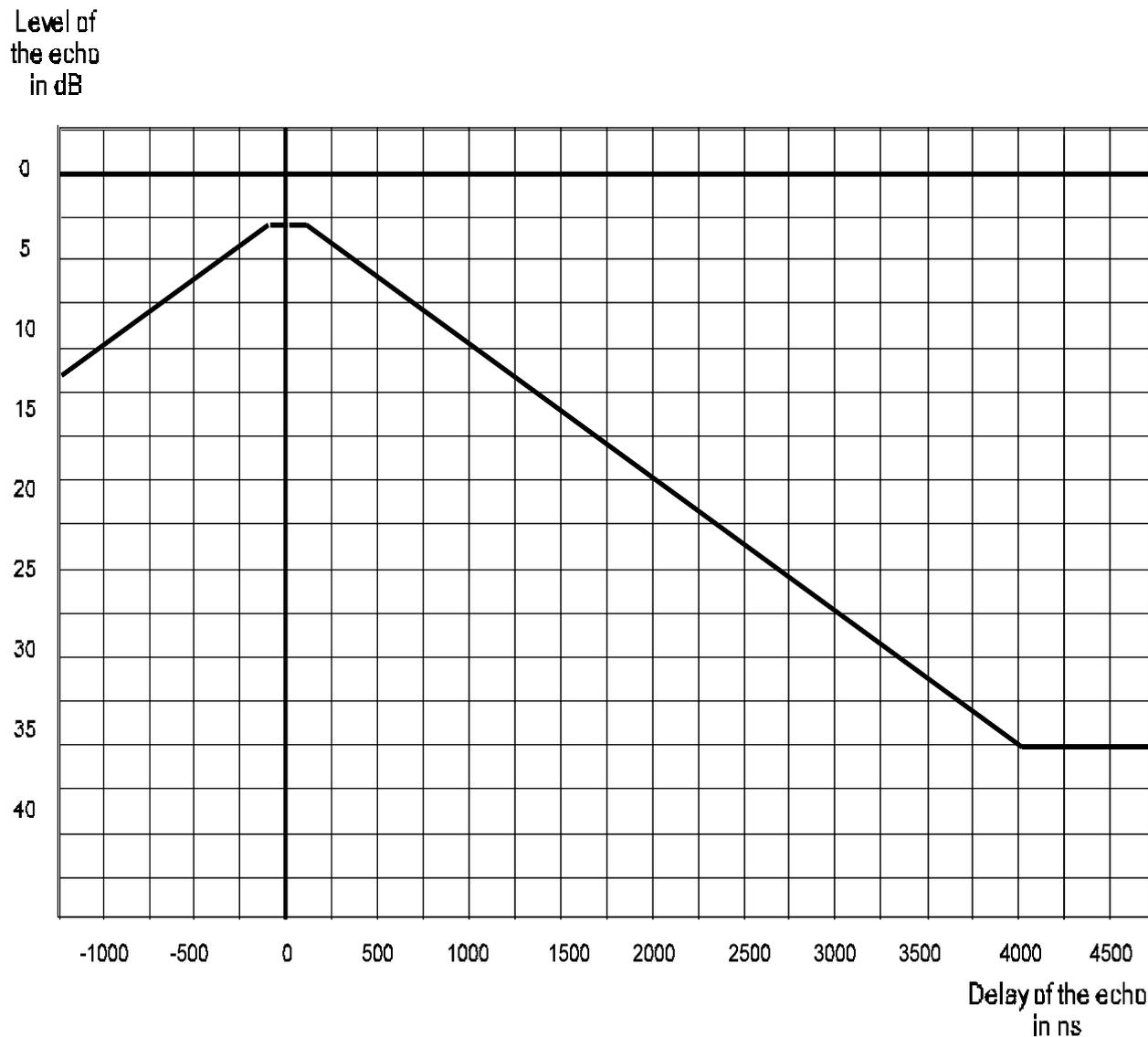
Figure B.14: Specification of an equalizer
