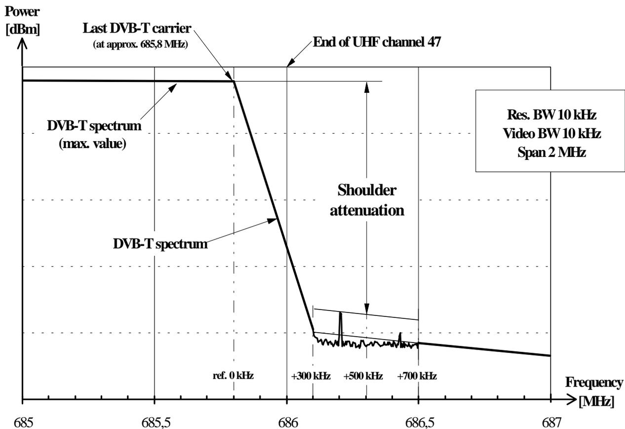
Figure E.9: Example with the upper edge of the DVB-T spectrum in UHF channel 47
