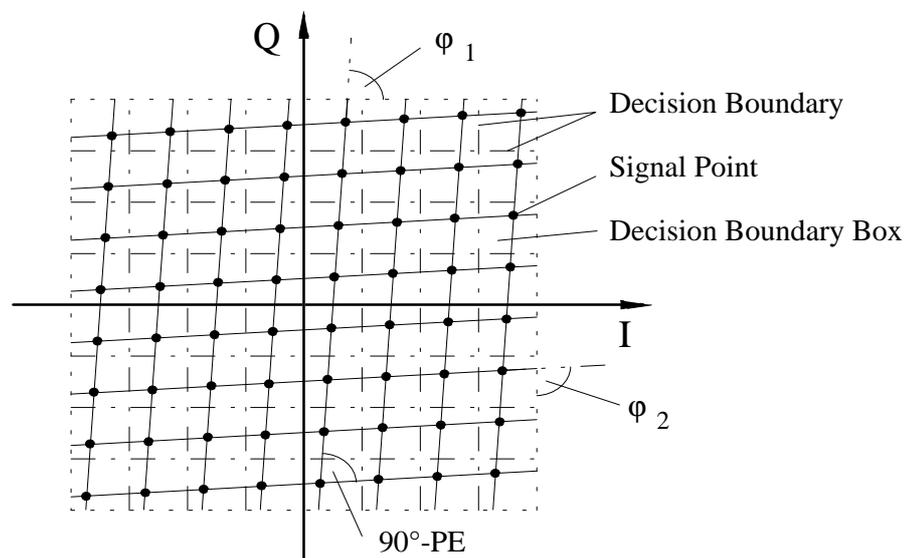
**Figure 17: Distortion of constellation diagram resulting from I/Q Quadrature Error (QE)**
