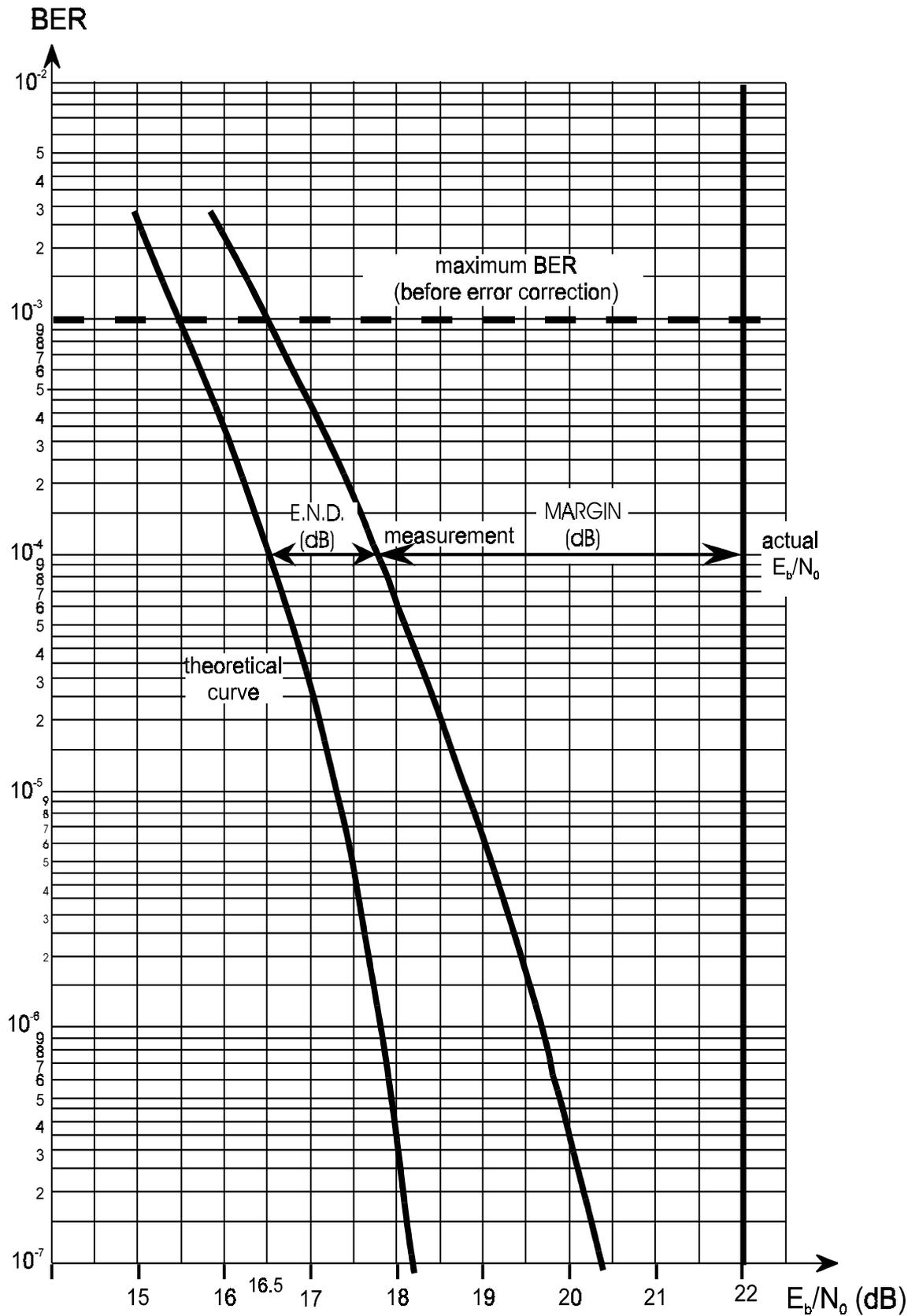
**Figure 10: Measurement of equivalent noise degradation**
