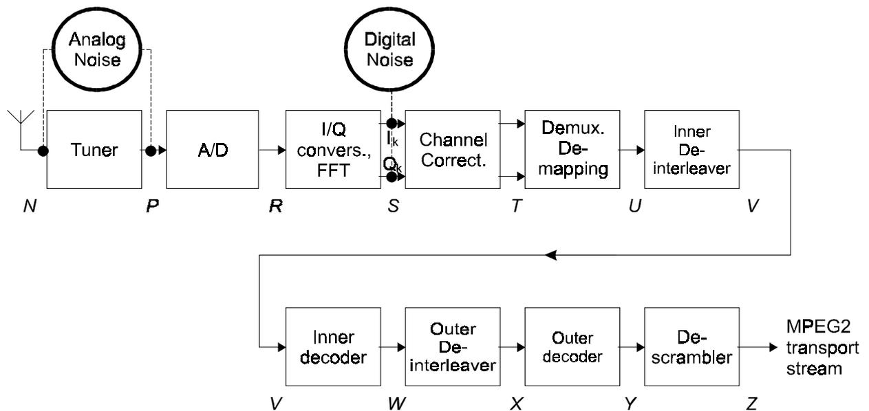
Figure 13: Block diagram of a DVB-T receiver
