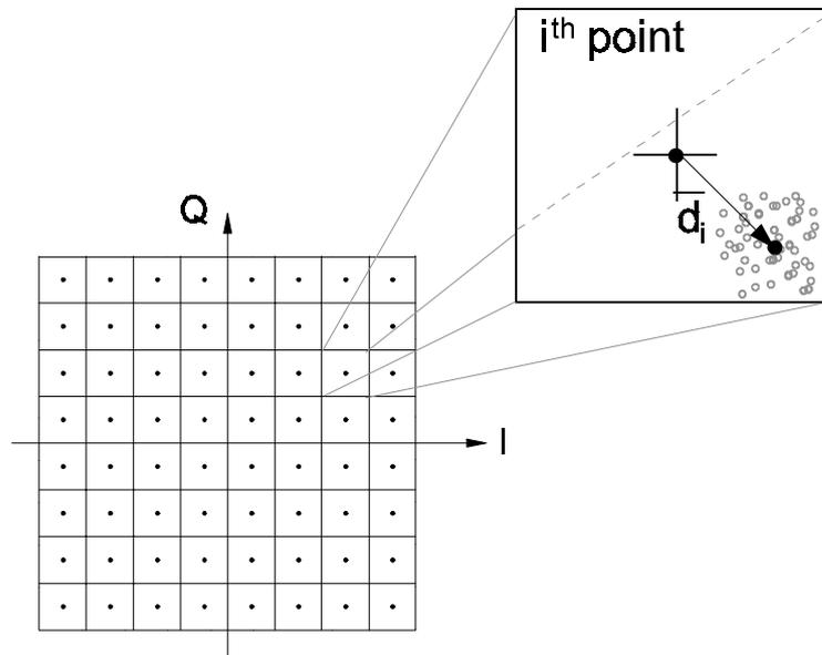
**Figure 6: Definition of Target Error Vector (TEV)**
