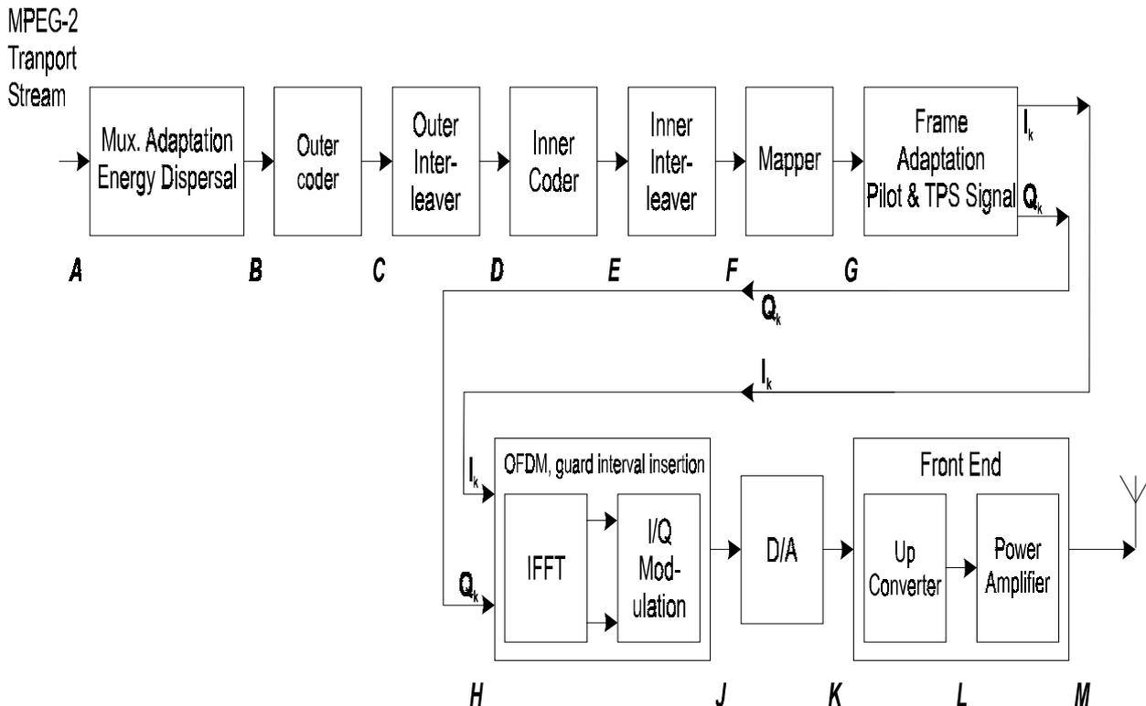
**Figure 12: Block diagram of a DVB-T transmitter**
