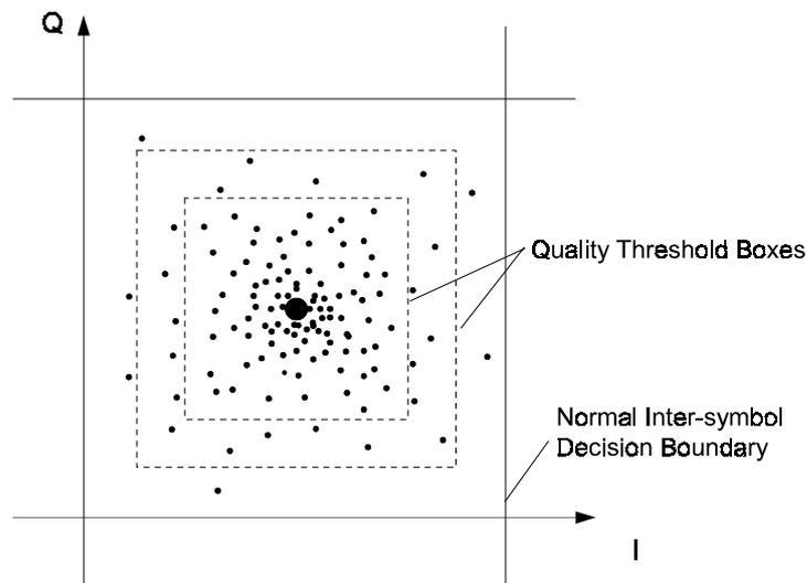
**Figure 9: Quality thresholds for single constellation in the I/Q plane**
