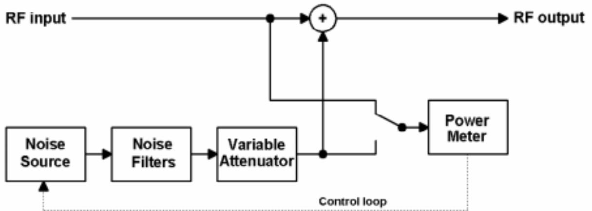
Figure G.3: Simplified block diagram of C/N test set
