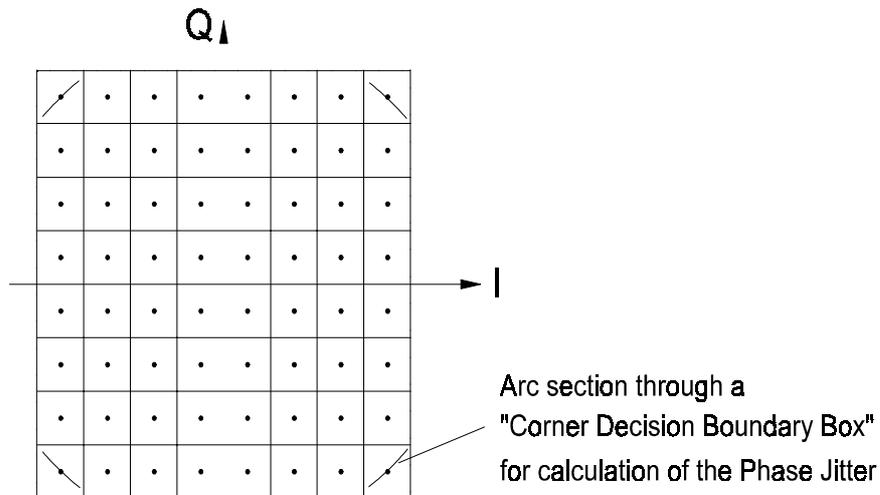
**Figure 8: Position of arc section in the constellation diagram to define the PJ (example: 64-QAM)**
