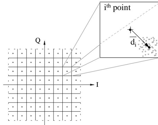
**Figure 16: Definition of Target Error Vector (TEV)**
